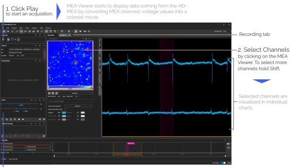
3. Chart window to adjust charts scale by dragging bars for time window width and for amplitude range.
