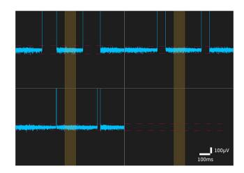
This behavior might be related to a wrong setting of the working point of the amplifiers that are integrated underneath the electrodes. In such case, follow the instructions below for a correct HD-MEA calibration; if the problem persists you can refer to the section <u>"Electrodes with no-signal (saturation)" P.38</u>.
