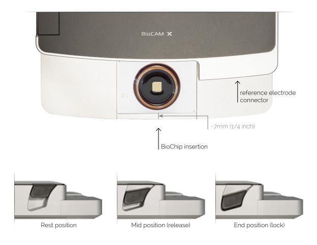
3. To start using the BioChip, plug the electrode reference into the BioCAM X and place the platinum end of the electrode inside the BioChip's reservoir, which must be filled in with a physiological saline solution (or a simple saline solution when performing system testings).
