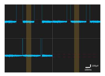
This behavior might be related to a wrong setting of the working point of the amplifiers that are integrated underneath the electrodes. In such case, follow the instructions below for a correct BioChip calibration; if the problem persists you can refer to the section <u>"Electrodes with no-signal (saturation)"</u>.
