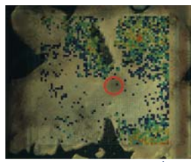
2.67 mm The neonatal mouse retina (P10) fits almost entirely on the electrode array.
